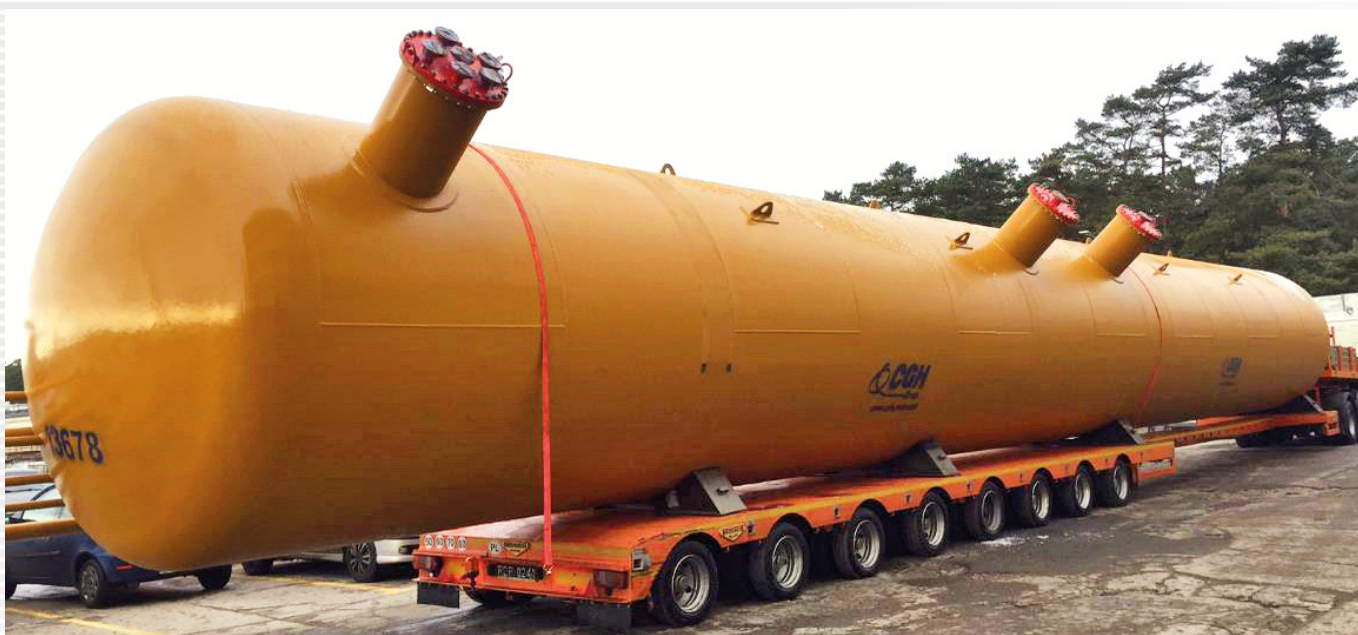
Project Baltic area, LPG Terminal: 3 x 200 m 3 , Ø 3200 mm
