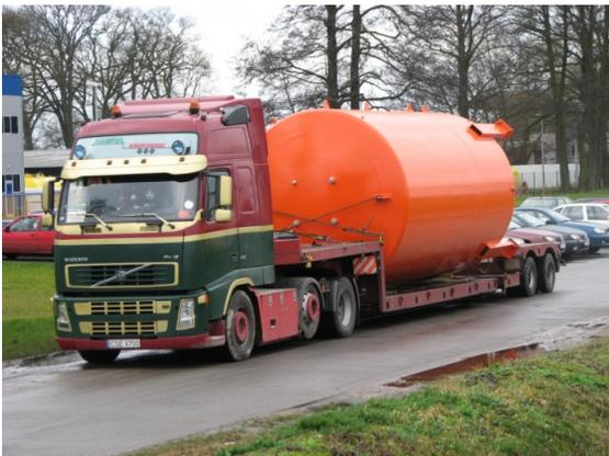
Special tank 51 m<sup>3</sup> diameter 3200 mm
