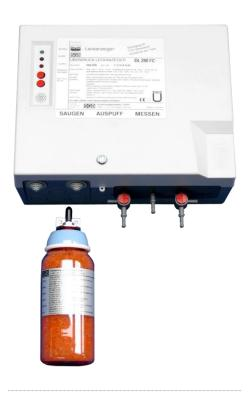
A leak prevention system to monitor double walled tanks. This model is equipped with an integrated dry filter sensor to indicate that the dry filter material is used. By this condensation and corrosion in the interstitial space can be avoided because a maintenance signal is indicated. Additionally this signal can be transferred via dry relay contacts.
