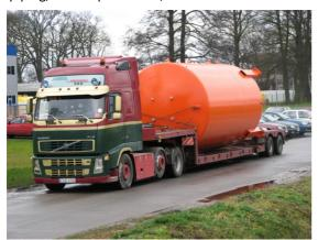
Special tank 51 m³ diameter 3200 mm
